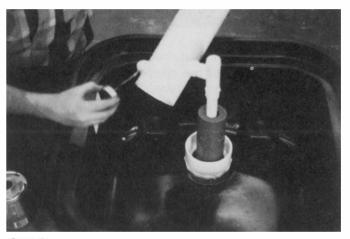
Step 8Using PVC pipe glue, glue the 4" pipe into the bottom fitting.\* NOTE (Important) PVC "T" is pointing toward the near left corner.
