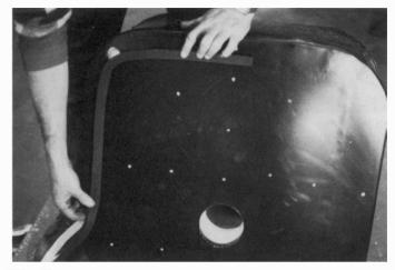
**Step 2**Stick the adhesive backed gasket to the bottom of the base assembly.
