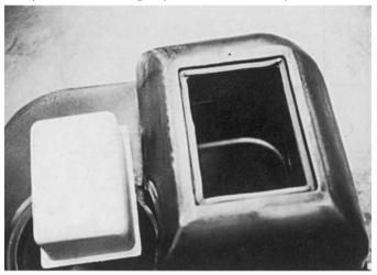
Install gasket material on the ledge inside the access hole. It is important that the gasket be installed here and not on the plug. Use a little grease on top of the gasket before putting in the plug. This makes it easy to remove the plug on cold days without damage to the gasket material.
