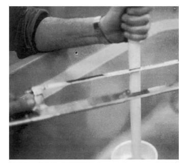
**Step 7**With a hack saw, cut off the fill line where you made your mark previously.
