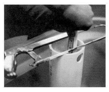
Step 5 With a pen or pencil, make a mark on the fill line 2 3/4" below the top of the 4" outer pipe.
