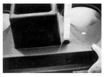
**Step 17** If you are dairy (dairy only) remove the 2 rubber plugs in the top portion of the tank. Then place the 3/4" pipe in the bottom hole. the 45° angle goes in the hole. Align so water can pass thru.
