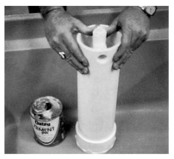
**Step 12**After PVC cement has been applied, push the riser pipe into the bottom fitting and align with the "T" fitting so the "T" fitting fits into the 1 1/4" hold at the top of the riser pipe. Push the 4" pipe down completely to the bottom of the fitting.
