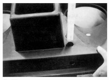
Step 18 If you are dairy (dairy only) remove the 2 rubber plugs in the top portion of the tank. Then place the  $^{3}/_{4}$ " pipe in the bottom hole. The 45° angle goes in the hole. Align so water can pass thru.
