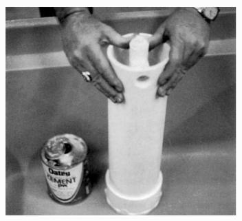
**Step 13**After PVC cement has been applied, push the riser pipe into the bottom fitting and align with the "T" fitting so the "T" fitting fits into the 1<sup>1</sup>/<sub>4</sub> hole at the top of the riser pipe. Push the 4" pipe down completely to the bottom of the fitting.
