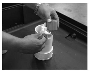
**Step 13** Apply teflon tape sealer to the valve threads.
