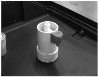
**Step 14**Screw the valve into the elbow so the valve is tight. In most cases, hand tight is sufficient. If wrenches are required, be careful not to over tighten.
