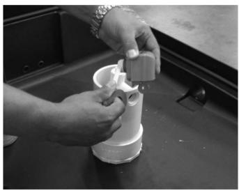
**Step 13** Apply teflon tape sealer to the valve threads.
