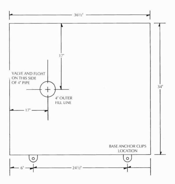
BECAUSE OF EXPANSION AND CONTRACTION OF THIS TYPE OF MATERIAL WE RECOM-MEND DRILLING ANCHOR BOLTS IN AFTER THE TANK IS SITTING ON THE CONCRETE PAD.
