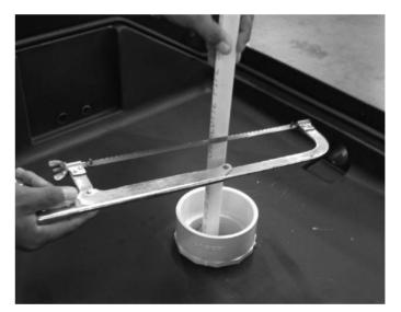
**Step 8**With a hack saw, cut off the fill line where you made your mark previously.
