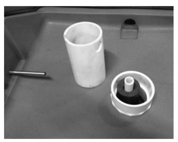
**Step 7**The riser pipe is not glued into the bottom fitting. Pull the riser pipe out of the bottom fitting.
