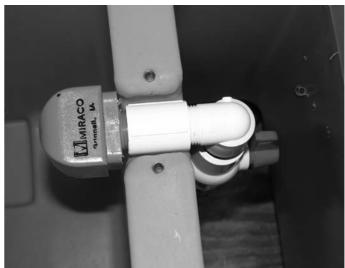
**Step 4**Set the entire assembly into the valve cradle.
