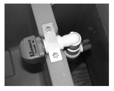
**Step 5**Place the stainless steel bracket over the PVC fitting and attach with 1/4" stainless steel screws provided.
