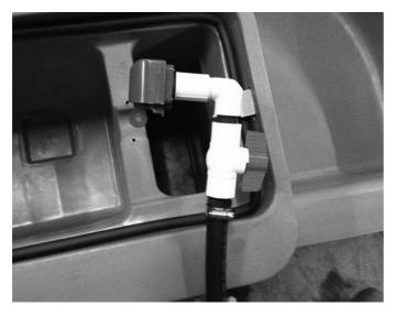
**Step 3**Attach the 150 psi hose with shutoff valve (provided) to the PVC elbow, use teflon tape on all threaded fittings.
