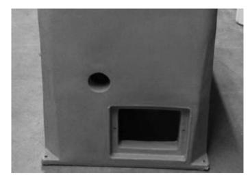
Access doors on each end for access to constant flow fitting on the bottom side of the tank. Constant flow drain pipes can be plumbed to drain on the ends or in the center. Center access door should be used for access to an approved electrical outlet for optional heaters.
