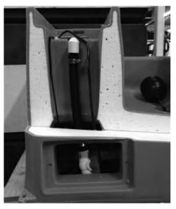
A 50 watt heat cabel is provided for your supply line to prevent freezing. Do not wrap on the line. Let the heat cord hang alongside the water line. Nylon zip ties are provided to hold heat string tight to water line.
